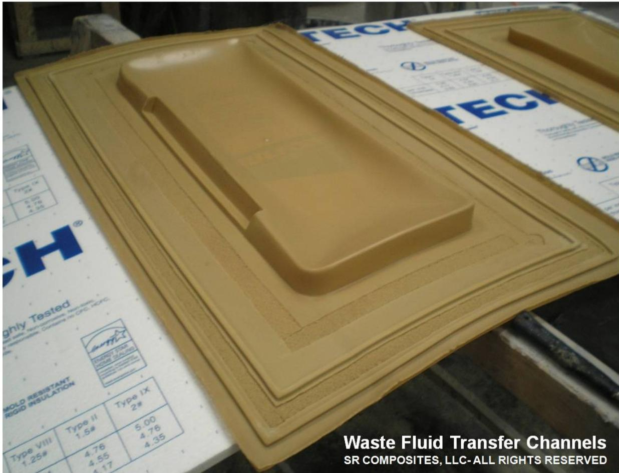
Figure 1: WFTC used as a Perimeter Seal and Reusable Vacuum Manifold in an RVB
