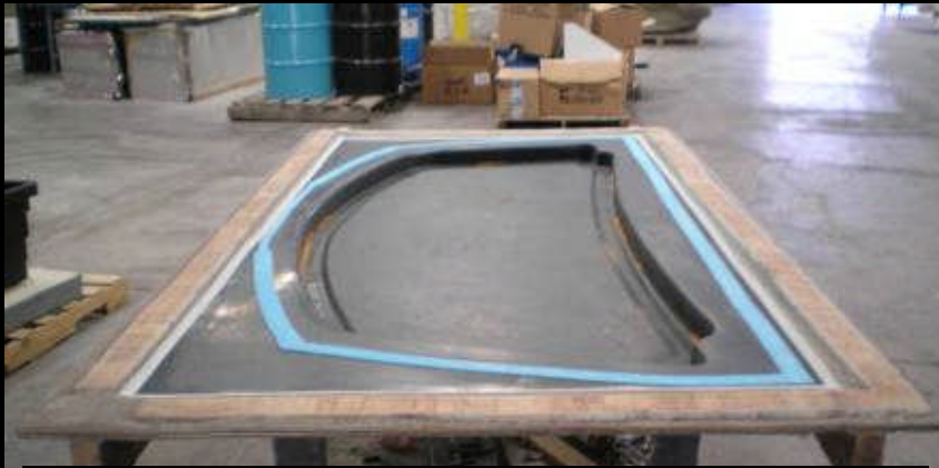
Mold Prep – Duratec Primer FRP Frame/Seal (taped inner edge) WFTC (Waste Fluid Transfer Conduit)
