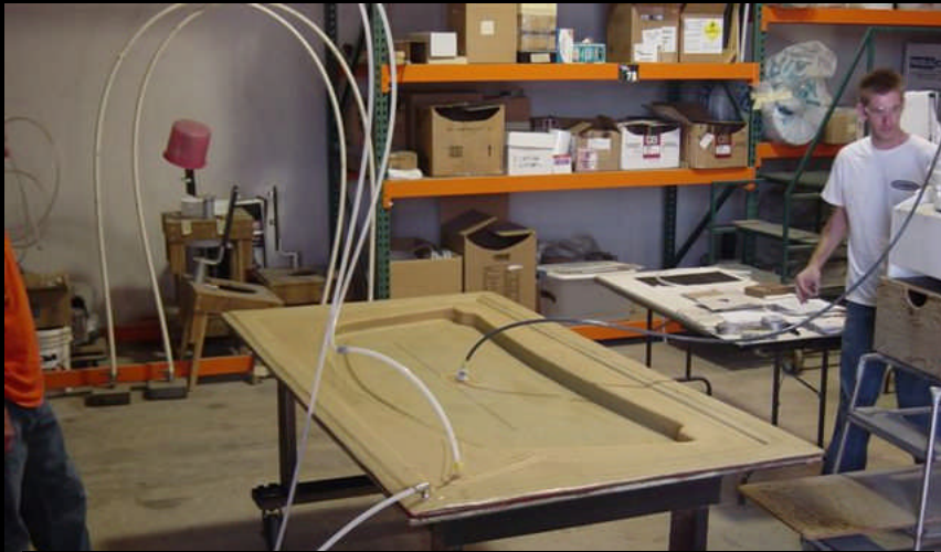
Frame Seal w/"D" Deals for Vacuum Single Point Resin Feed - Infusion
